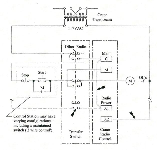
If Radio Power is to be separate from Main Power, omit jumper from C (Main) to X1 and add Transfer Switch contact with dashed line connection as shown.
